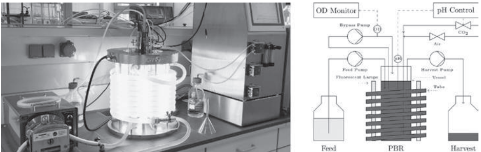
Fig. 1. Experimental set-up; left : xCubio PBR (bbi Biotech); right : Outline of the experimental chemostat set-up (adapted from Weise et al. [2]).
